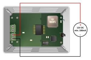
**Important:** If a wired remote controller of the Indoor Unit manufacturer is connected to the same bus, communication may shut down. Connect the PS connector of AC Cloud Control to an external power supply to overcome this situation.
