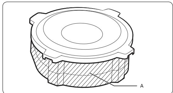
Insulate the end of the pipe and some curved area by using separate insulator.
