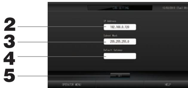
2. **Setting and viewing the IP Address (Factory default: 192.168.0.120)**
