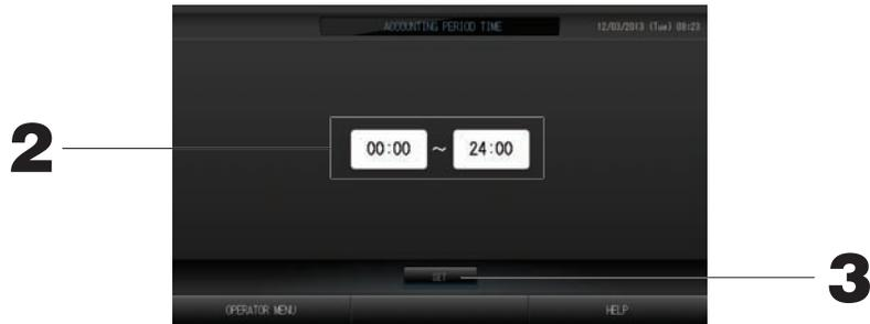
2. Press the hour or minute buttons for the start time or the end time.
