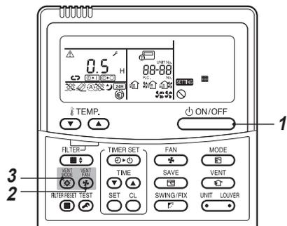
**1** Push the buttons to start operation. The operation lamp lights up.
