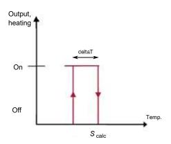
Figure 2-2 Heating function
