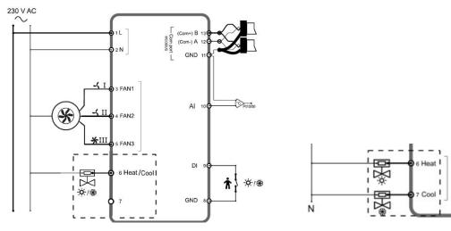
Figure 4-1 2-pipe wiring (standard)
