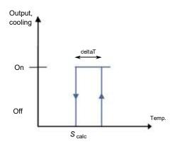
Figure 2-3 Cooling function
