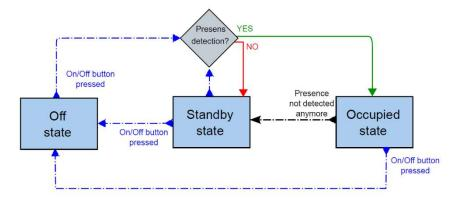
Figure 2-11 Changing controller states (no remote control)
