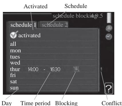
When scheduling is active the relevant blocking symbol is shown in the main menu on the symbol for the control module.
