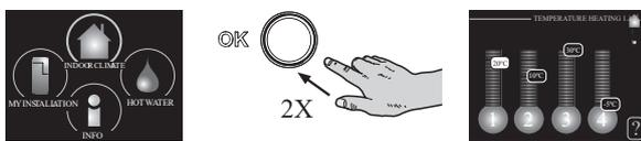
The mode for setting the indoor temperature is accessed by pressing the OK button twice, when in the start mode in the main menu. Read more about the settings on page 14.
