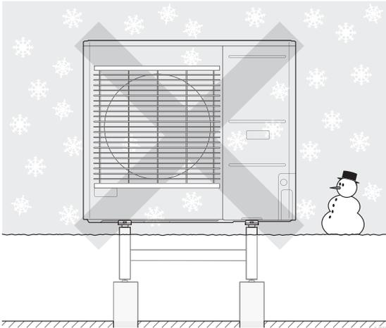
Prevent snow from building up and covering the grilles and drain holes on FDCW.
