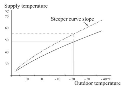
The optimum slope depends on the climate conditions in your location, the type of heating device (radiators or under floor heating) and how well insulated the house is.
