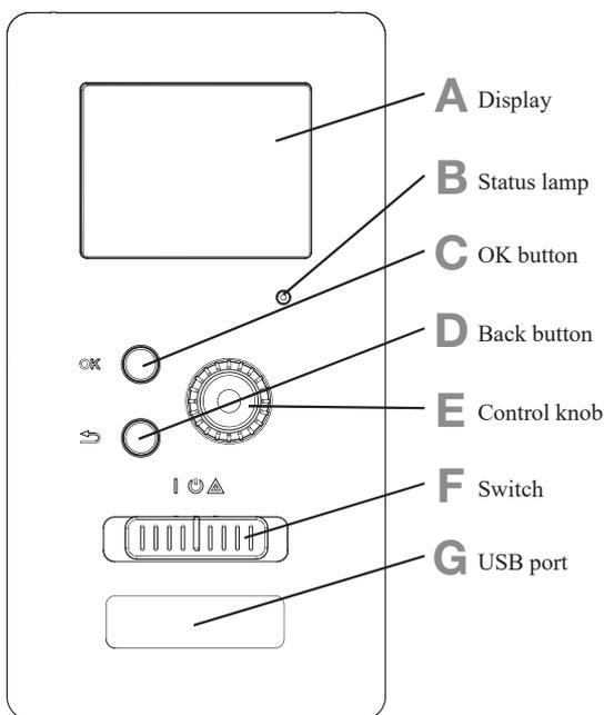
There is a display unit on the front of the control module, which is used to communicate with RC-HY20/40. Here you:
