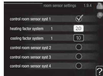
\*If there is one climate system, display shows "control room sensor system 1" only.
