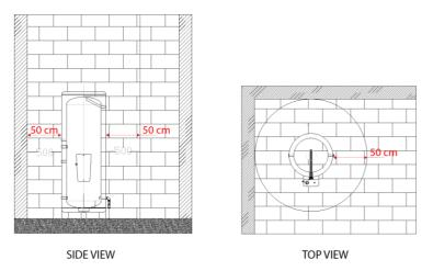
b) For maximum performance, install the DHW tank in frost free places.
