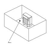
B) Install in a space with a depression height of ≤ 0.1 [m].
