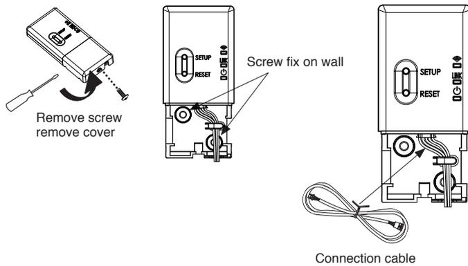
4. Insert lead wire in to unit and connect Wi-Fi terminal.
