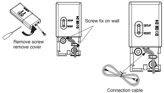
3. Insert lead wire in to unit and connect Communication cable.
