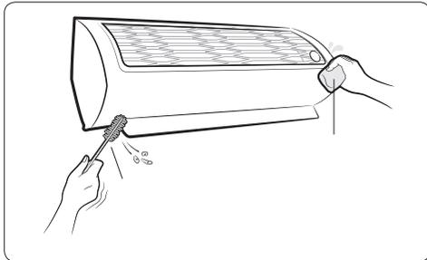
Wipe the surface of the unit with a slightly wet or dry cloth when needed. Wipe off dirt from oddshaped areas by using a soft brush.
