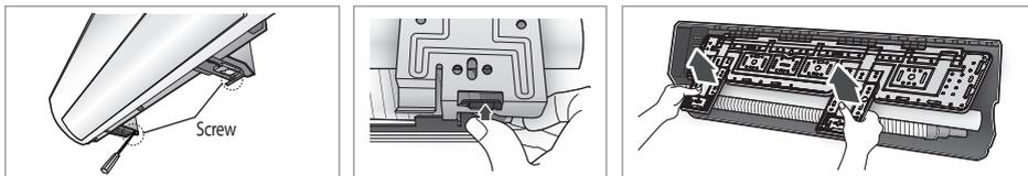
3. Determine the position of the pipe and drain hose hole as seen in the picture and drill the hole with an inner diameter of 65 mm so that it slants slightly downwards.
