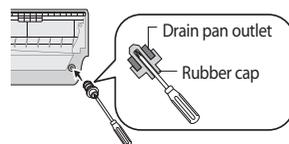
Pour the water in direction of arrow. \* Direction of the drained water
