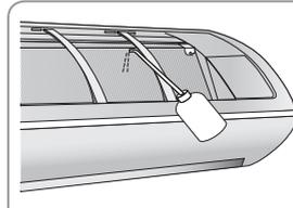
After completing the installation of the drain hose, pour water into the drain pan to check whether the hose is well drained.
