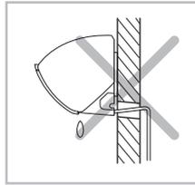
The drain hose must NOT slant upwards.
