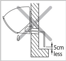
Keep a clearance of at least 5 cm between the end of the drain hose and the ground.
