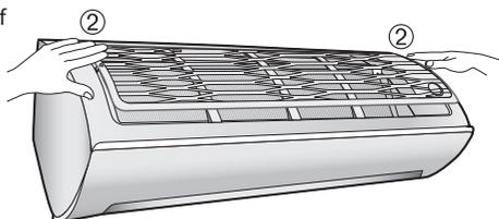
3. Press the bottom of the filter lightly to securely fix the main body. ③④⑤
