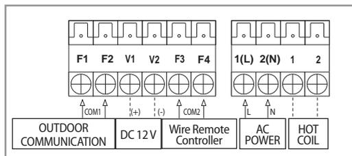
\* The output of hot coil terminal is AC 220 V / 230 V
