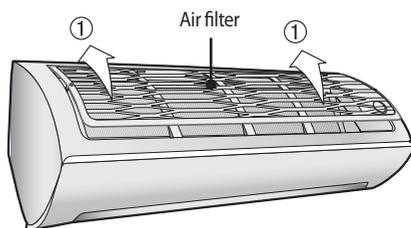
2. There's one hook in both side of the filter, press the surface of the Air filter softly and get the hooks into the main body. ②
