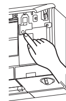
Emergency operation switch (E.O. SW)
