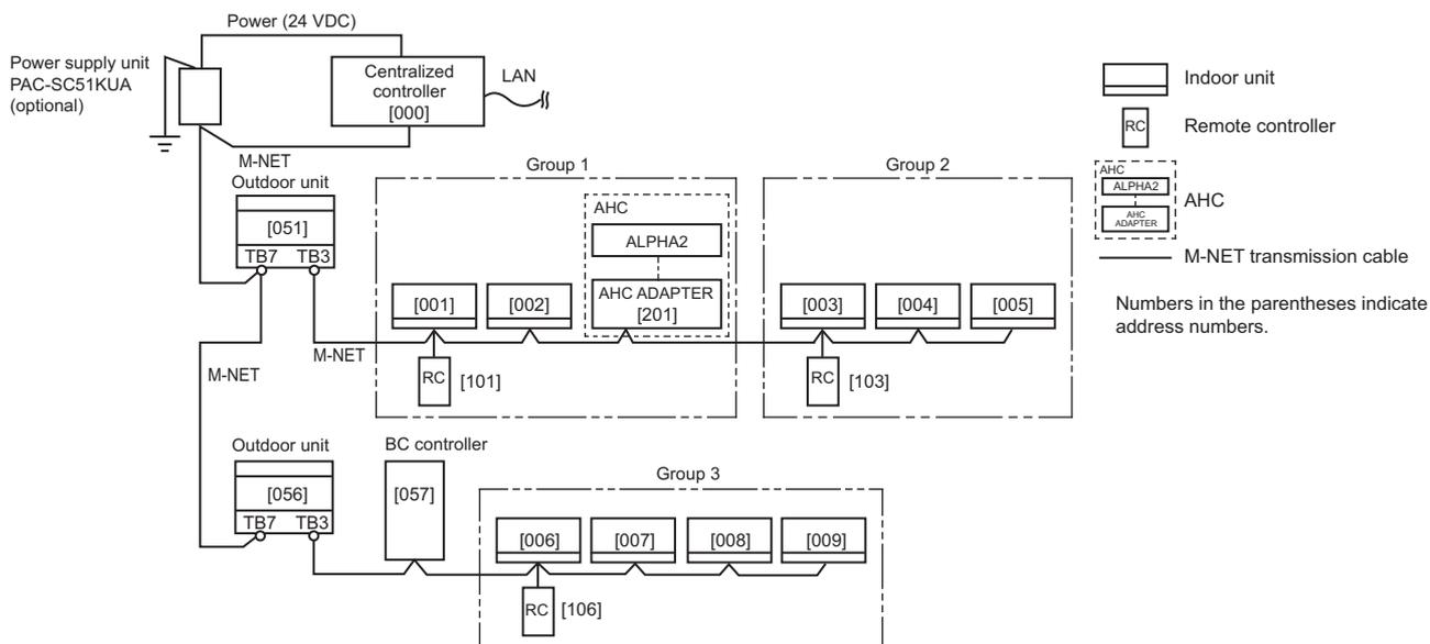
\* AHC ADAPTER requires either an outdoor unit or a power supply device as a power source.
