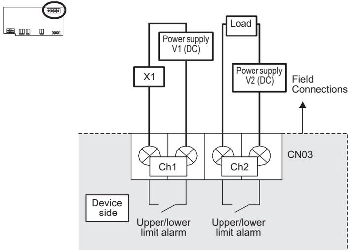
Tightening torque for terminal screws: 1 N·m.
