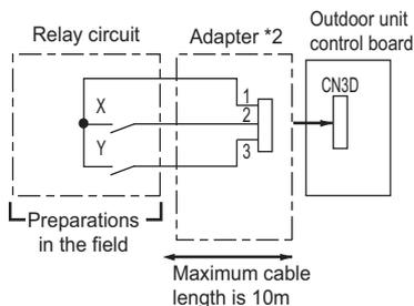
X, Y : Relay Contact rating voltage  $\geq$  15VDC
