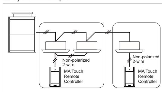
\*When a PAR-CT01MA is connected to a group, no other MA remote controllers can be connected to the same group.
