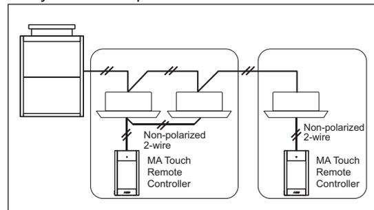
\*When a PAR-CT01MA is connected to a group, no other MA remote controllers can be connected to the same group.
