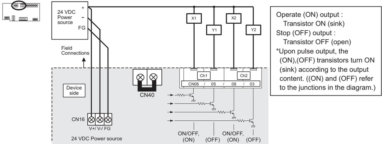
Tightening torque for terminal screws: 1 N·m
