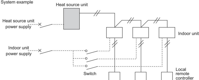
Restart of the CITY MULTI needs to be careful. When no power supply to the heat source unit, no power supply to the compressor case heater too. The compressor needed to be warmed up before running. When using above functions, power supply to the heat source unit should be ensured.
