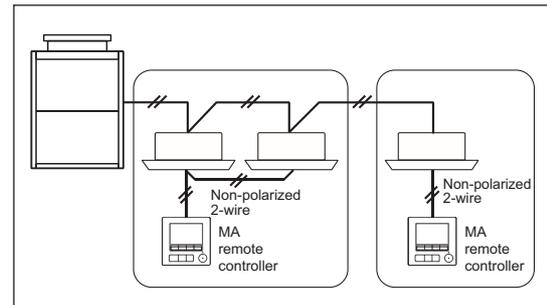
\*When a PAR-40MAA is connected to a group, no other MA remote controllers can be connected to the same group.
