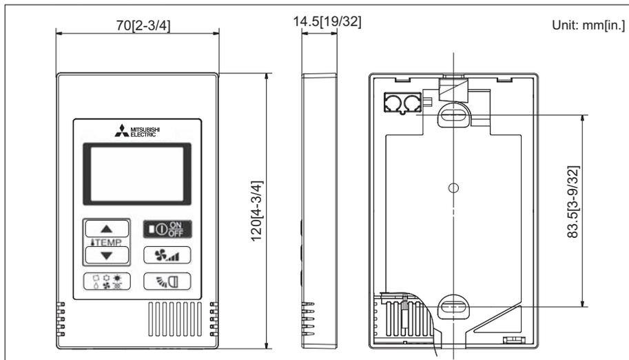
2-7. Wireless remote controller [PAR-FL32MA/PAR-FA32MA/PAR-SL100A-E/PAR-SE9FA-E/PAR-SF9FA-E/PAR-SL94B-E]
