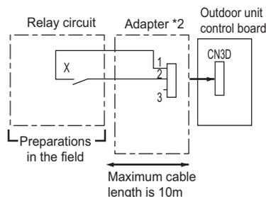
X: Relay Contact rating voltage  $\geq$  15VDC
