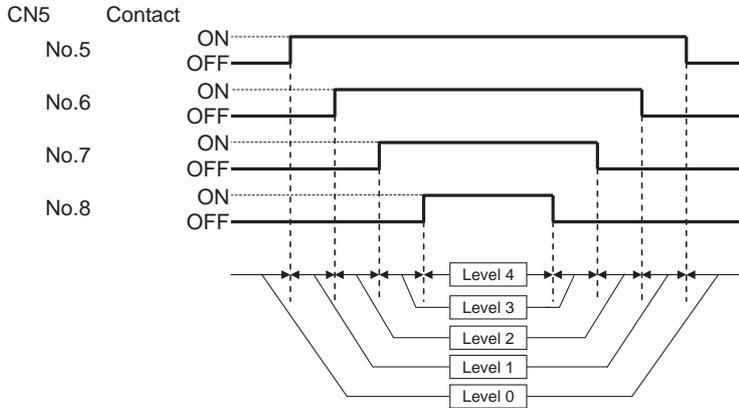
Demand level signal specification: Only the current levels' contacts turn on.
