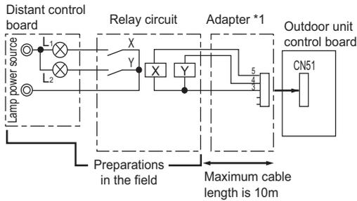
L1 : Heat source unit error display lamp
