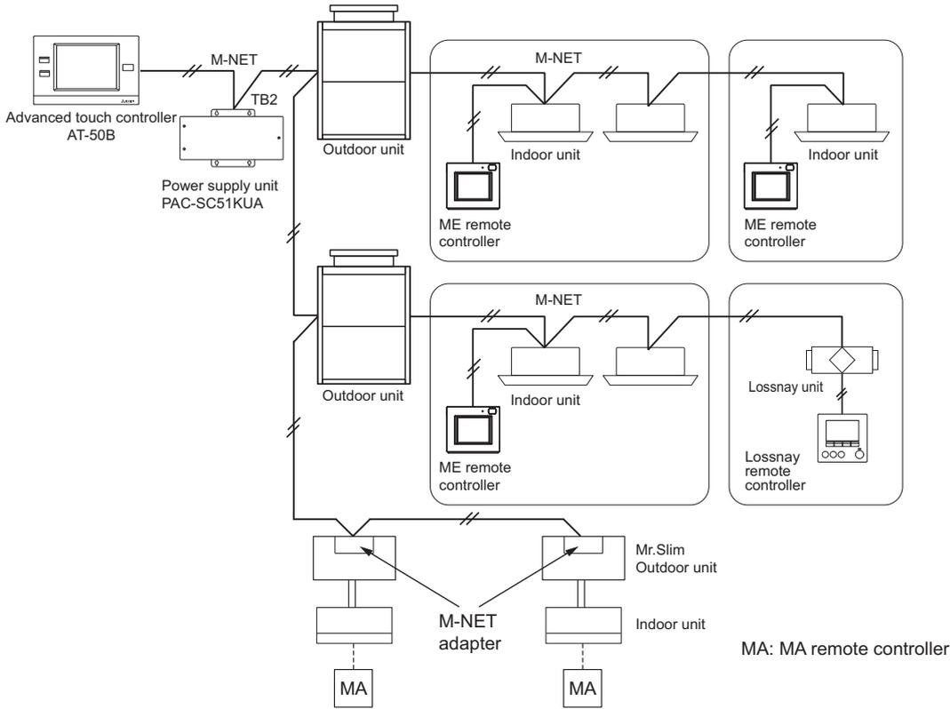
Fig. 1 Basic structure of AT-50B and PAC-SC51KUA
