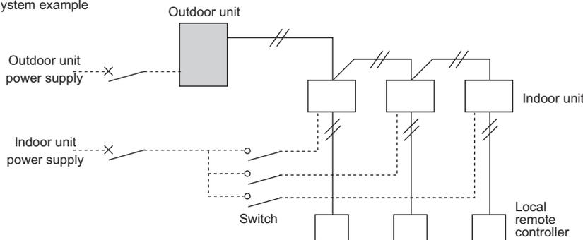
Restart of the CITY MULTI needs to be careful. When no power supply to the outdoor unit, no power supply to the compressor case heater too. The compressor needed to be warmed up before running. When using above functions, power supply to the outdoor unit should be ensured.
