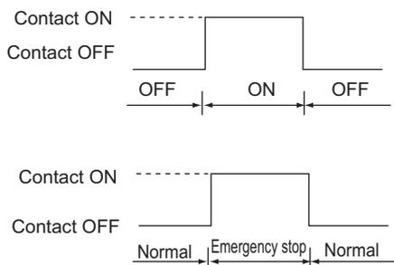
(B) Pulse signal (Example) for ON/OFF
