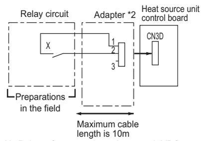
X : Relay Contact rating voltage  $\geq 15VDC$
