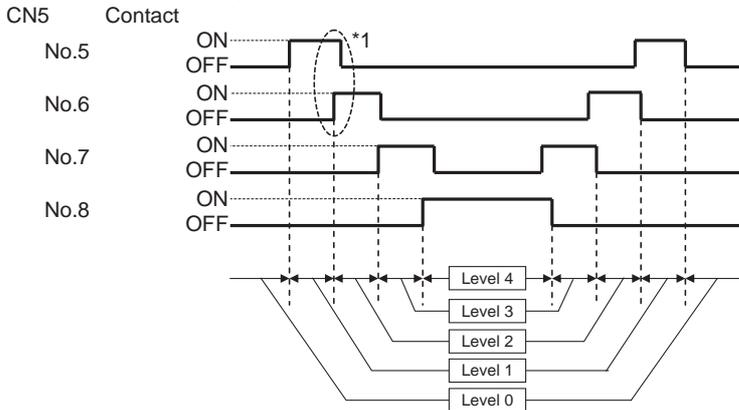
\*1 The specification must be followed in the following order: ① When the level changes, the contact of the level after the change turns on.; ② The contact of the level before the change turns off.
