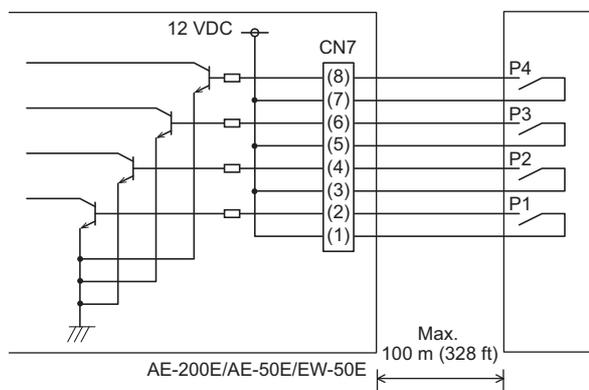
A voltage of 12 VDC is applied to CN7. Do not apply a power voltage from any other power source.
