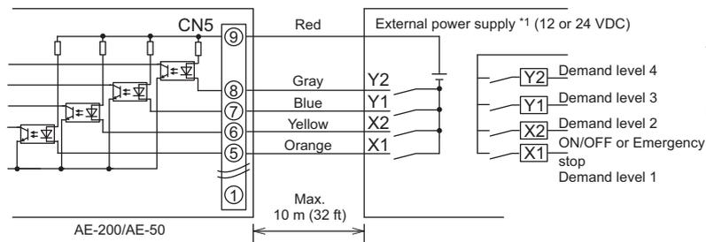
Use relays X1, X2, Y1, and Y2 that meet the following specifications.
