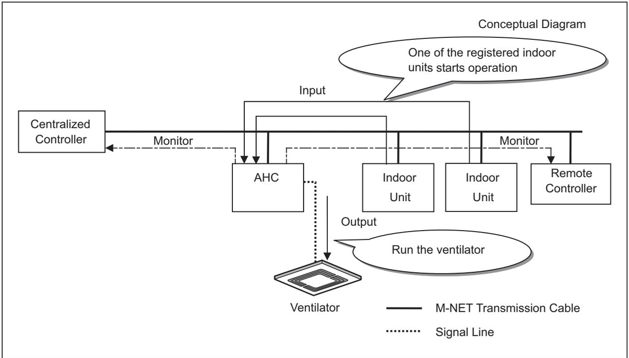
**Interlocking the Heater, Humidifier, and Fan**
