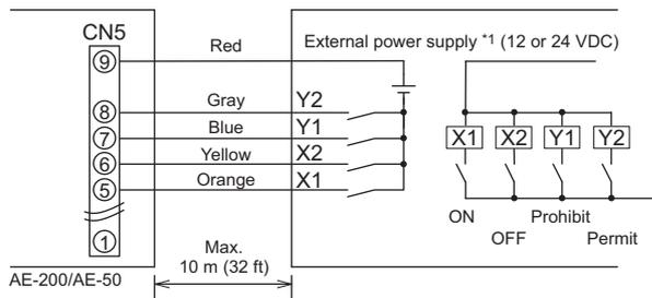
\*1 Select an external power supply suitable for the relays used. (12 or 24 VDC)
