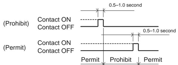
1. If the input pulse signal is the same as the current operation status of the air conditioning units, no status change will occur. (For example, if an ON signal is input while the air conditioning units are in operation, the units will continue their operation.)
