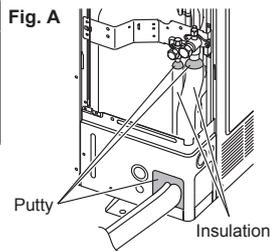
If the outdoor unit is installed at a level that is higher than the indoor unit, the water that has condensed in the 3-way valve of the outdoor unit could travel to the indoor unit. Therefore, use putty in the space between the pipe and the insulation to prevent the entry of water to the indoor units.
