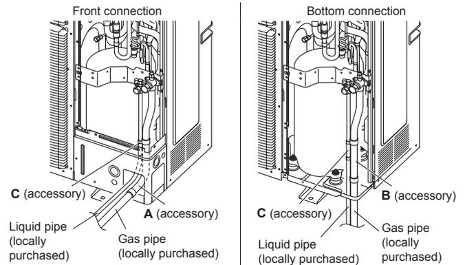
**A:** Joint pipe A (090 model), Joint pipe A-L (108/126/144/162 model)
