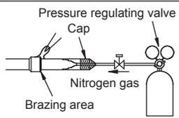
If a pipe is brazed without applying nitrogen gas, it will create an oxidation film. This can degrade performance or damage the parts in the unit (such as the compressor or valves).
