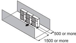
**When an obstruction is present also in the upward area** Unit: mm
