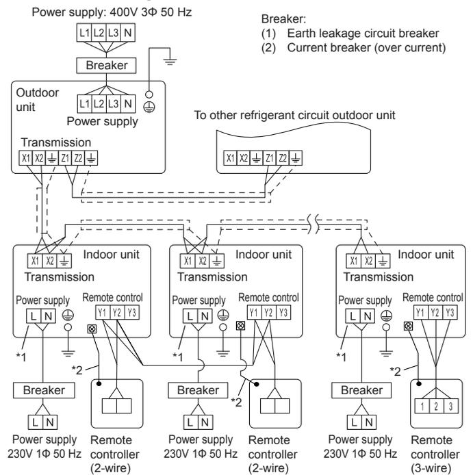
\*1: The number of power supply terminals is different depending on the indoor unit model. For the wiring, refer to the indoor unit installation manual.
