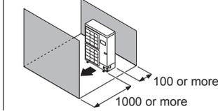
**When an obstruction is present also in the upward area** Unit: mm
