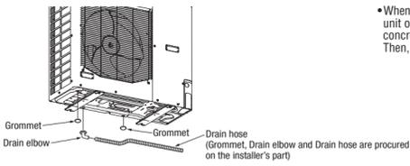
When condensed water needs to be led to a drain, etc., install the unit on a flat base (supplied separately as an optional part) or concrete blocks. Then, please secure space for the drain elbow and the drain hose.
