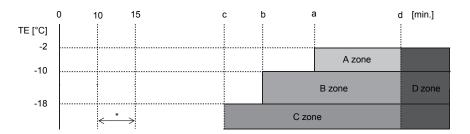
\* From 10 minutes to 15 minutes after a heating operation started, the minimum value of TE is stored in memory as TEO and the minimum temperature of TO as ToO.
