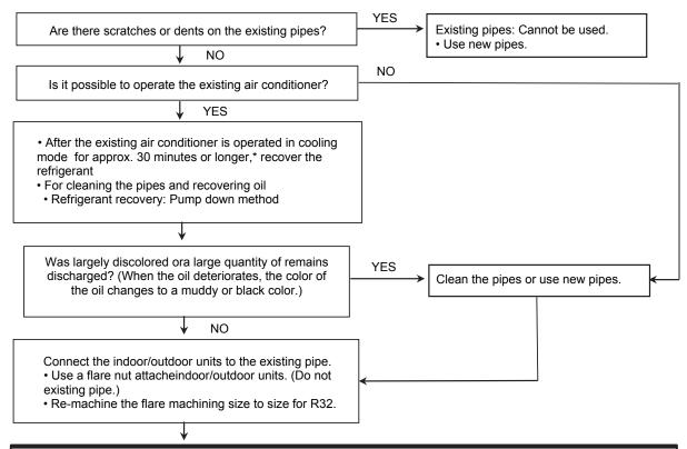
■ In case use existing pipe,The gas pipe Ø19.1 mm is able to use for the outdoor unit of GM80 (3 Hp) or higher,However, Prior specify to use gas pipe Ø19.1 mm. for the air conditioners
