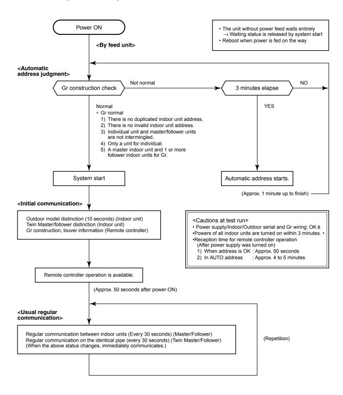
In a group operation, if the indoor unit which was fed power after judgment of automatic address cannot receive regular communication from the master unit and regular communication on identical pipe within 120 seconds after power was turned on, it reboots (system reset).
