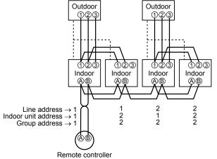
For the above example, perform setting by connecting singly the wired remote controller without remote controller inter-unit cable.
