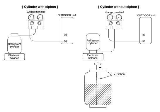
Fig. 6-4-2 Configuration of refrigerant charging when using a cylinder equipped with/without a siphon
