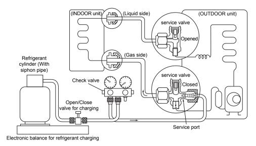
Fig. 6-4-1 Configuration of refrigerant charging
