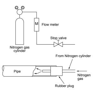
Fig. 6-5-1 Prevention of oxidation during brazing
