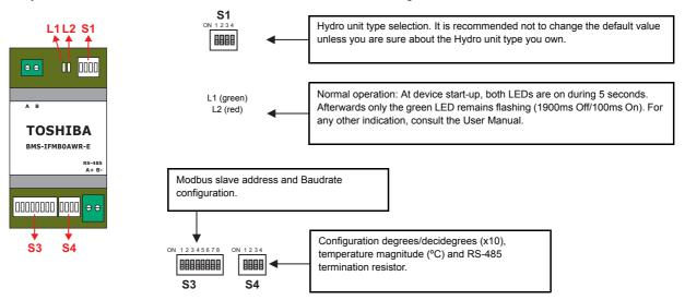
The following table applies for configuration of the interface through these DIP-switches:
