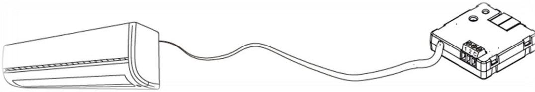
**Figure 2.** Connecting KLIC-DD v3 to the A/C unit.
