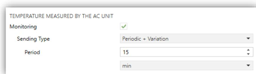
Figure 8. AC Gateway. Configuration. Temperature measured by the AC unit.
