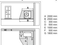
4) Protective zone for wall installation in front of a building wall
