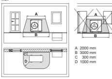
3) Protective zone for ground installation in a building corner
