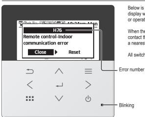
Below is a list of error codes that may appear on the display when there is some trouble with the system setting or operation.
