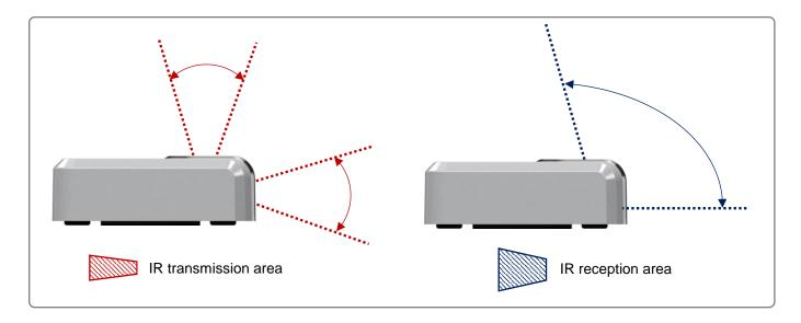
Figure 3.1 IR emitters and IR receiver location
