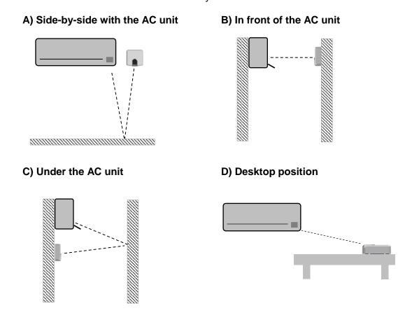
Figure 3.2 IR emitters and IR receiver location
