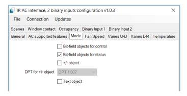
Figure 5.6 AC mode additional communication objects
