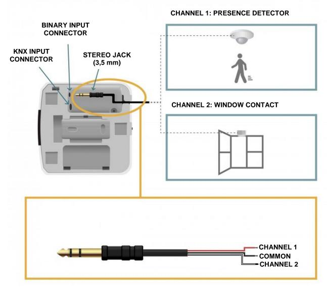
Figure 3.7 Binary Input connection
