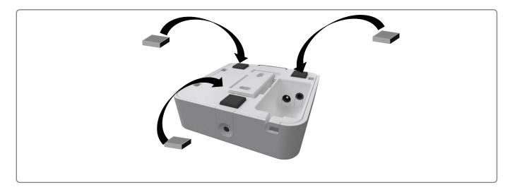
Figure 3.4 Rubber dumpers location
