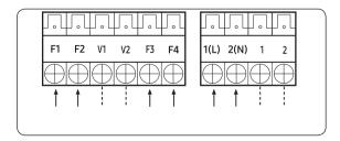
$\star$  The output of hot coil terminal is AC 220 V / 230 V
