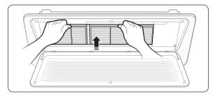
To assemble the air filter, proceed in reverse
