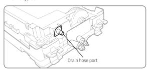
**3** Cover the flexible hose with the provided insulation drain.
