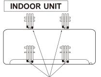
Wet and dry bulb thermometers FRONT VIEW
