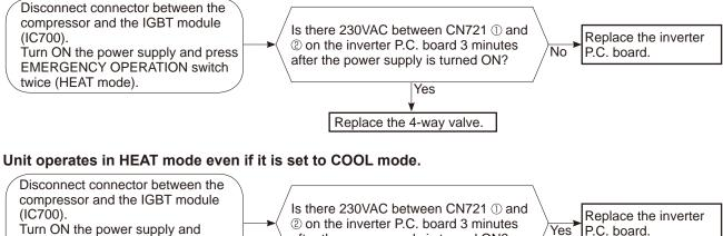
Turn ON the power supply and press EMERGENCY OPERATION
